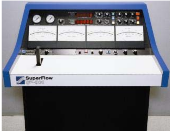
The engine dynamometer used at L&M Engines is a Superflow SF 901
