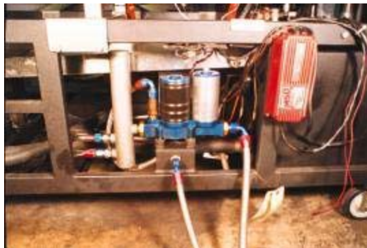
Fuel Pump & Filter
